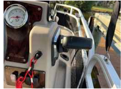
Throttle: neutral in the middle; trim button on handle
