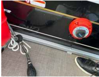
Battery switch: set to ALL
