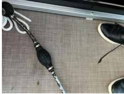
Primer bulb on the fuel hose: squeeze to re-prime
