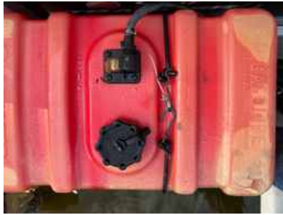
Fuel tank & gauge (top of the red tank)
